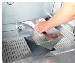
Mount the filter cassette and the strainers
