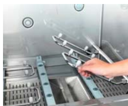
Fold the lower rinsing pipes upward
