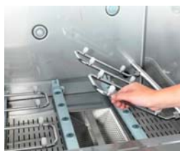
Fold the lower rinsing pipes downward
