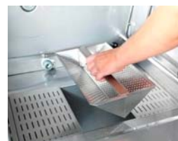
Remove the filter cassette and the strainers
