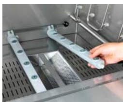
Remove the lower wash arms and if necessary, clean them
