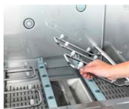
Fold the lower rinsing pipes downward
