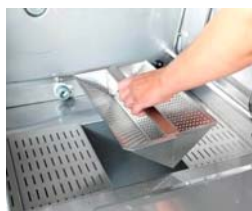
Remove the filter cassette and the strainers
