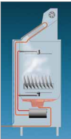
Schematic diagram of the heat recovery process in the GS 640 Energy (only possible with cold water connection)
